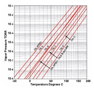
One vapor-diffusion pump oil cannot meet all the requirements of the various pumps in use. For example, for large scale pumps a robust, medium high vacuum oil is required; for high vacuum work a high quality, stable, very low vapor pressure fluid is needed; for general laboratory use there is a need for a relatively inexpensive low vapor-pressure fluid. To cover these various requirements, several grades of Apiezon vapor-diffusion pump oils are available.
