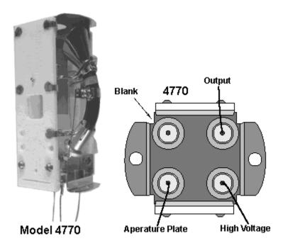
Four styles of multipliers are used on all models of Hewlett Packard mass spectrometers.
